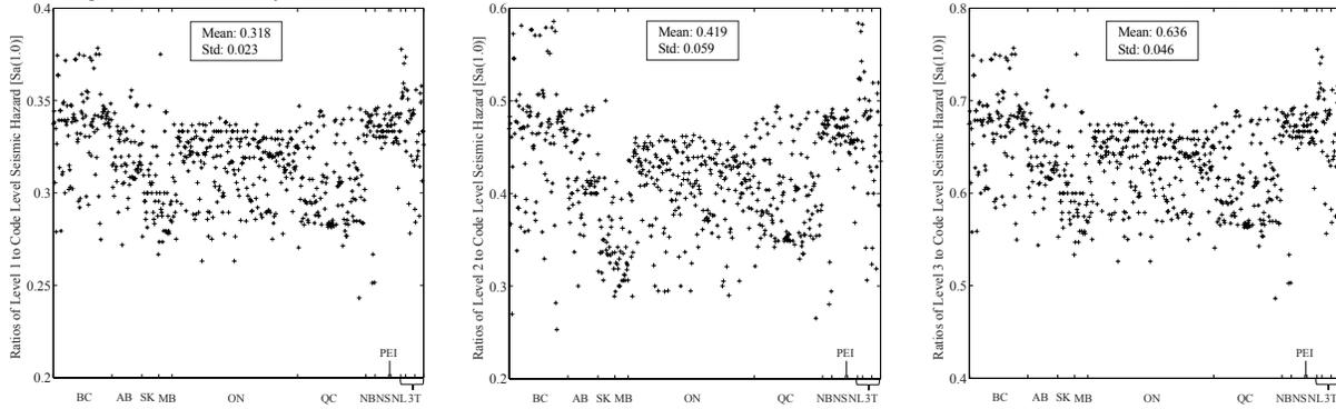
Figure 4: Ratios of Level 1, Level 2, and Level 3 seismic hazards to Code Level seismic hazard [ $S_a(1.0)$ ]
