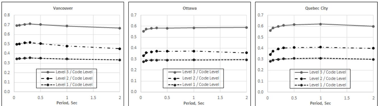
Figure 6: Ratios of Reduced Seismic Hazard Levels to Code Level Seismic Hazard for Vancouver, Ottawa, Quebec City
