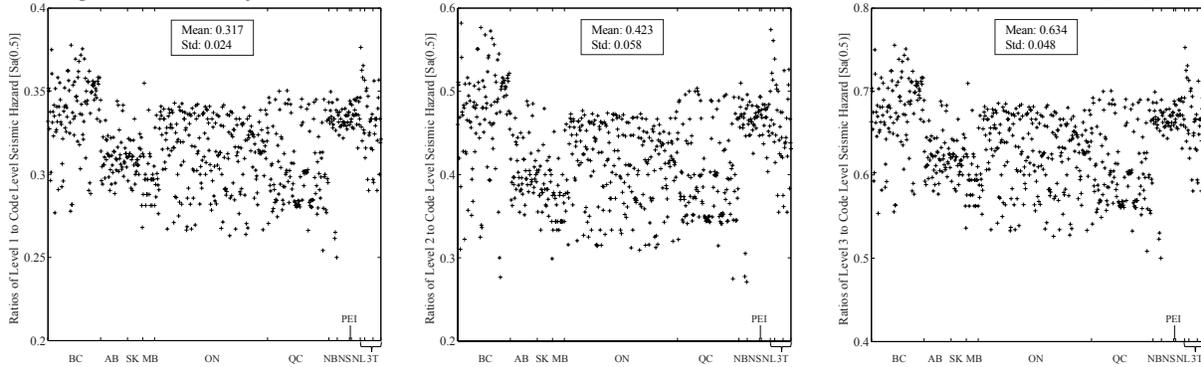
Figure 3: Ratios of Level 1, Level 2, and Level 3 seismic hazards to Code Level seismic hazard [ $S_a(0.5)$ ]
