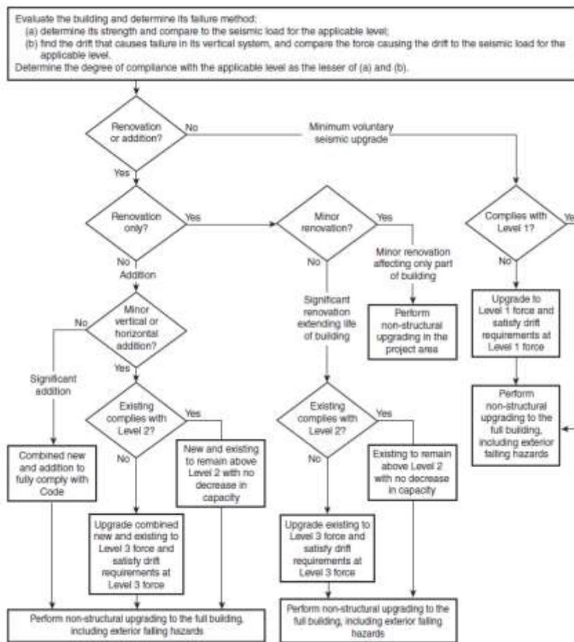
Figure 1 Flowchart for seismic assessment and upgrading of existing buildings (From Commentary L of the NBC 2015 [4]).
