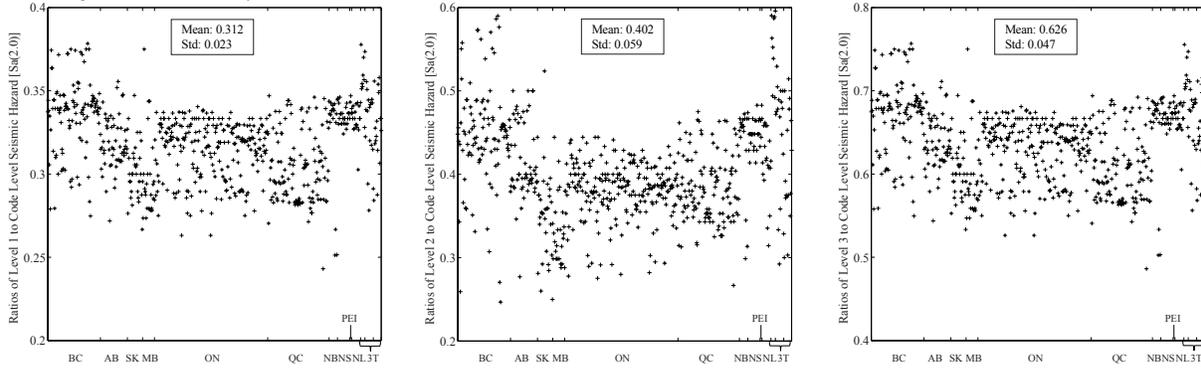
Figure 5: Ratios of Level 1, Level 2, and Level 3 seismic hazards to Code Level seismic hazard [ $S_a(2.0)$ ]
